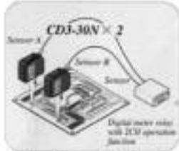
Detection of Warp in Circuit Board
