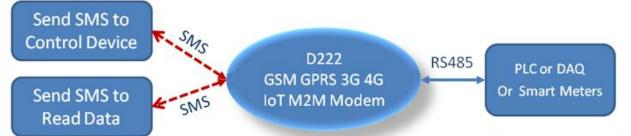
E.g.: Use mobile phone to control special device or read meter via SMS. So send the PLC's or meter's Commands by SMS to the PLC or Meter, like Modbus RTU Commands. After the PLC or meter response data to serial port, the D222 will forward to Mobile phone by SMS.
