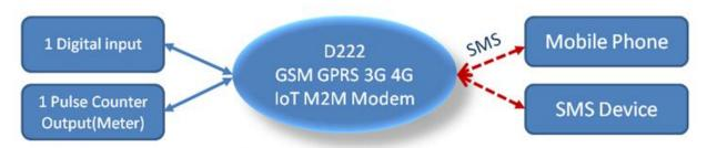
E.g.: Use for monitoring 1 digital input or pulse counter, while active or the counter reach the preset value, will send SMS to users' mobile phone.
