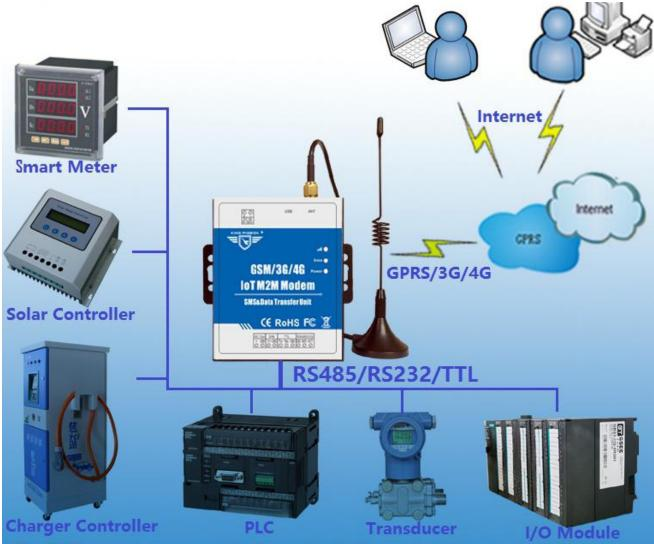
The D223 provides a secure, high speed, reliable wireless data transmission between Com port and internet connection for customer over GPRS/3G/4G wireless cellular network, it can be used as SMS modem and Modbus RTU to Modbus TCP converter.
